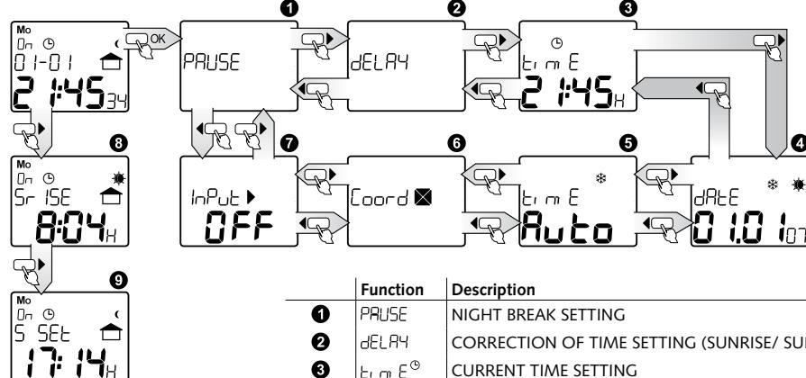
Enter the menu from the main window by choosing OK; move inside menu using cursors ▲▼. Return to the main window is possible after pressing button ⌚ or ⌚.
